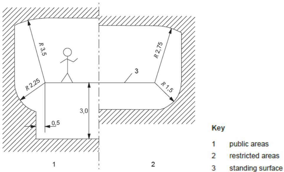
**Figure 4-4: Minimum clearances to accessible live parts on the outside of vehicles as well as to live parts of overhead contact line systems from standing surfaces accessible to persons for high voltages (EN 50122-1)**
