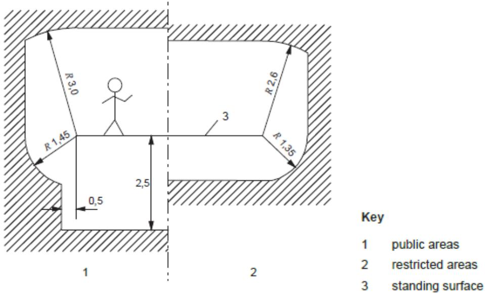
**Figure 4-3: Minimum clearances to accessible live parts on the outside of vehicles as well as to live parts of overhead contact line systems from standing surfaces accessible to persons for low voltages (EN 50122-1)**
