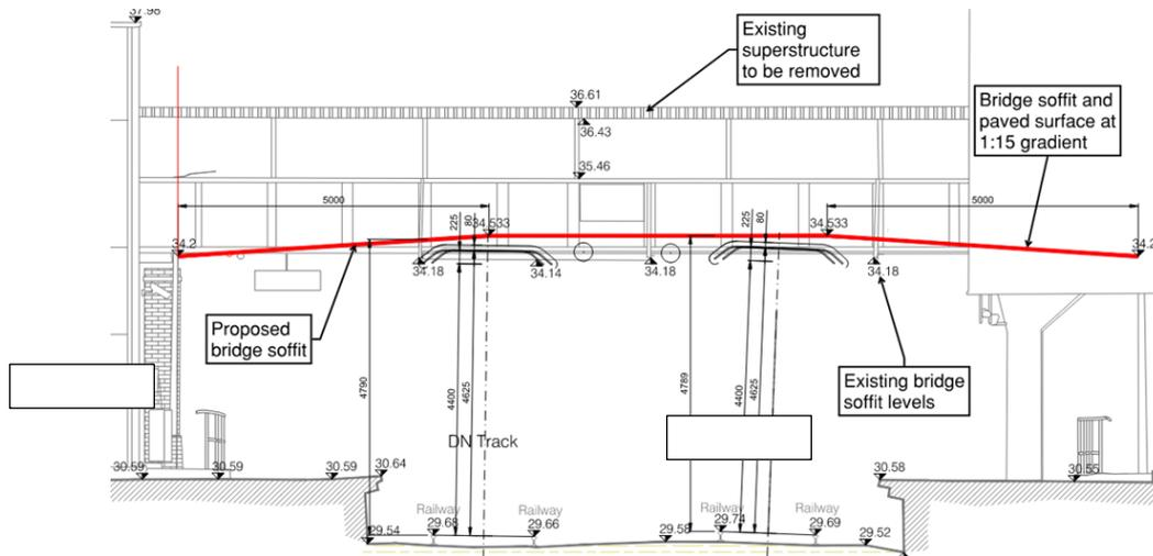
**Figure 4-1: Elevation of proposed superstructure replacement at OBB81**
