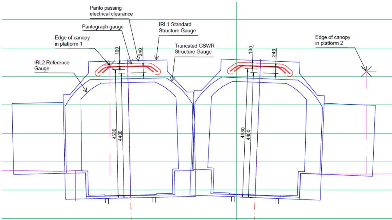
**Figure 5-1: Cross section through the north end of the platform canopy**
