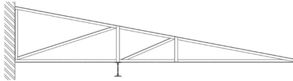
**Figure 5-8: Intermediate Truss (nts)**
