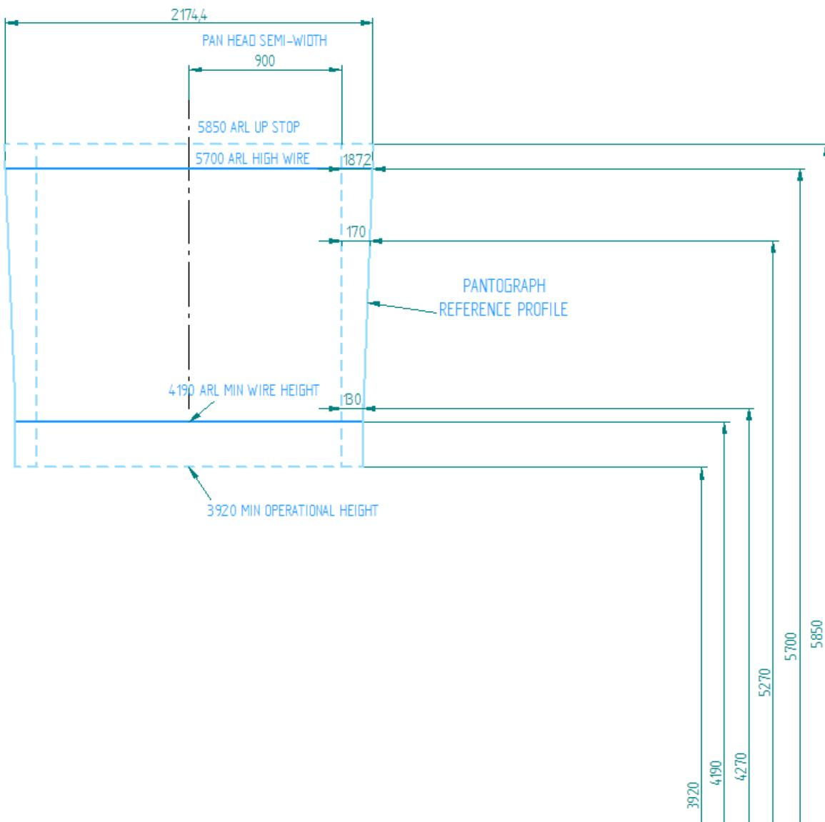
Figure 4-5: Reference profile for pantograph gauge given in the standard CME-TMS-327 – Vehicle Gauging
