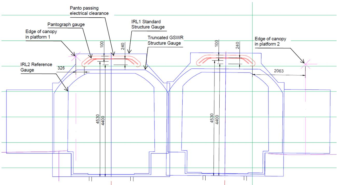
**Figure 5-2: Cross section through the south end of the canopy**
