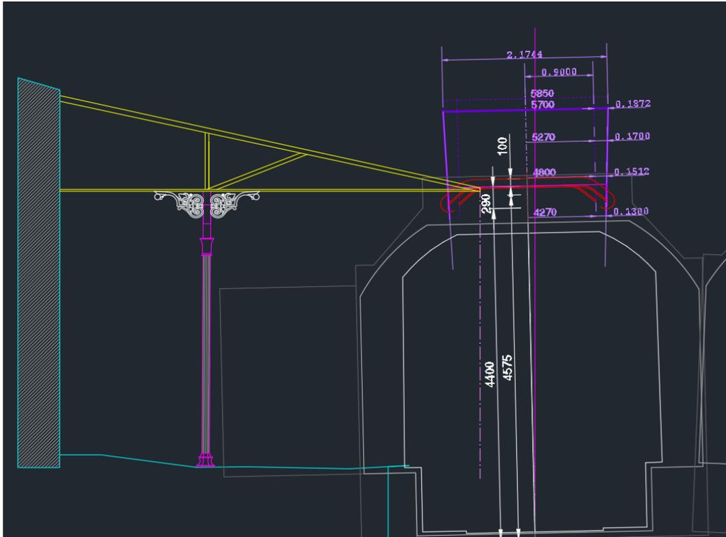
Figure 5-10: Platform 1 Cross Section Canopy compared to Pantograph reference profile
